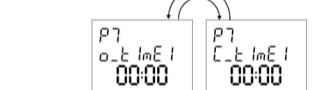
P7 Menu Navigation (Menu refers to program entry for 5 pairs of ON/OFF times.)
