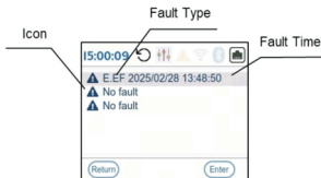
Figure 2.7.3 Fault log page
