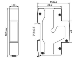
Fig.2 External and mounting dimensions
